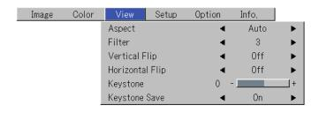
Each press of the SELECT ▶ button advances the selection one step in the sequence of "Color" → "View" → "Setup" → "Option" → "Info." → "Image". Each press of the SELECT ◀ button causes a return of one step.
