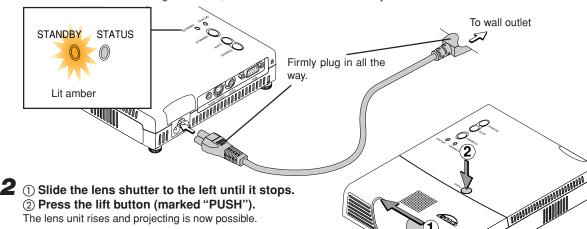
Switch on the projector power Press the STANDBY button.
