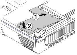
(2) Turn the lamp cover's screw clockwise to tighten it.
