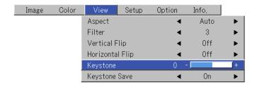
Adjustment display: Each press of the button results in a change of 1 point and continued presses cause changes to proceed in order.
